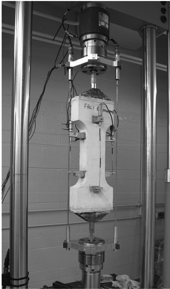
Fig. 2—"Dog-bone" test setup.
