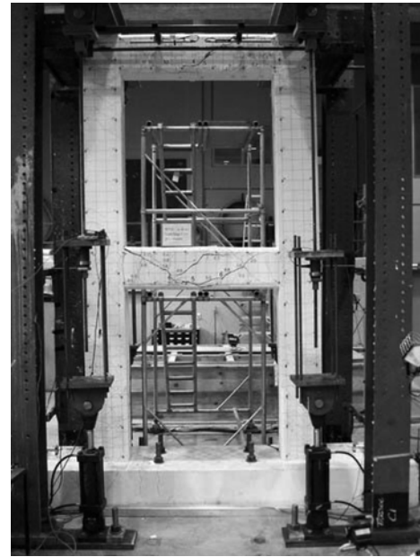
Fig. 14—Overall frame deformation at peak reverse half-cycle (Phase A).
