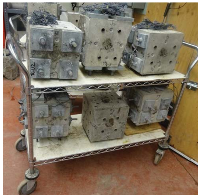
Fig. 1—Cube specimens with different stress states being stored on a cart.
