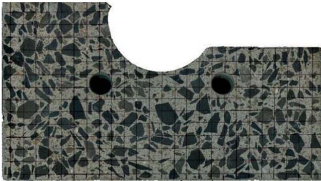
Fig. 3—DRI slice from biaxial specimen along XY plane at 8 months of accelerated curing (grid size is 1 x 1 cm [0.4 x 0.4 in.]; length is 254 mm [10 in.]).
