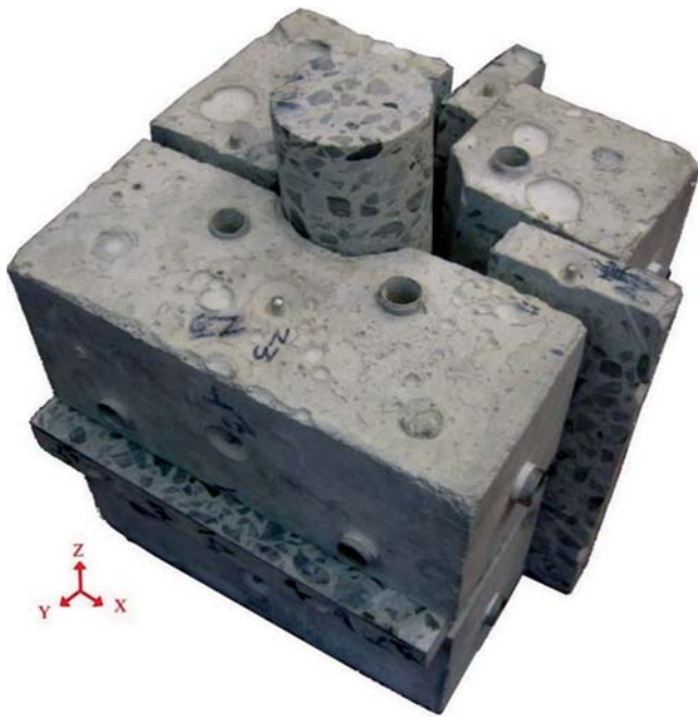
Fig. 2—Dissection of no-stress cube specimen (254 mm [10 in.] size) along three mutually perpendicular planes (YZ, ZX, and XY) for DRI analysis and core-drilled along Z-axis.
